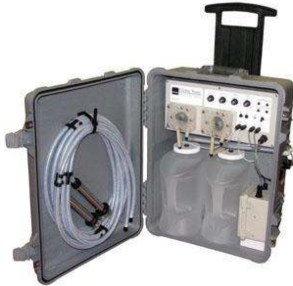
Figure 6: Inside of an autosampler
